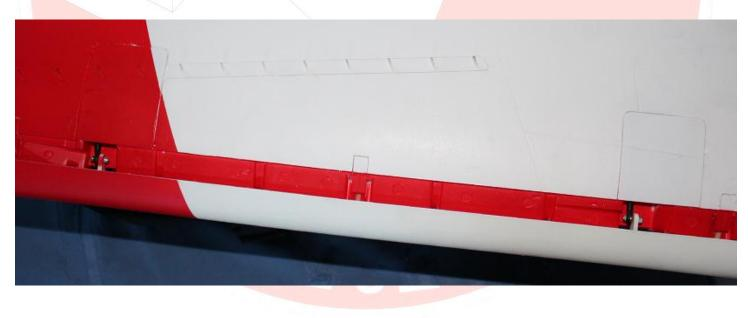
The servos are covers are glued and you would have to pry them out, I have removed them here to show you how they are installed at the factory.
