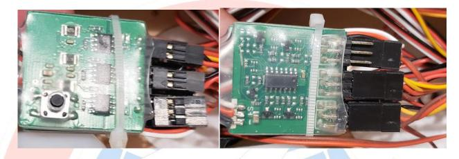
There are two main brake controllers used, a JP basic brake controller and the AG-63 Gyro Assisted Brake controller. The AG-63 will stop your jet by applying brakes and help correct steering if the airplane is not tracking strait (if your airplane is sliding or drifting). We have been using the AG-63 Exclusively in our personal jets and highly recommend this product.
