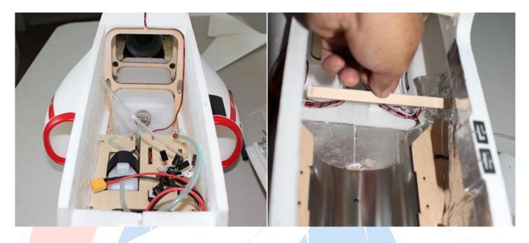
The main tank is held in place with a wood stopper, assemble the three pieces of wood and secure them with CyA to hold your main tank in place.
