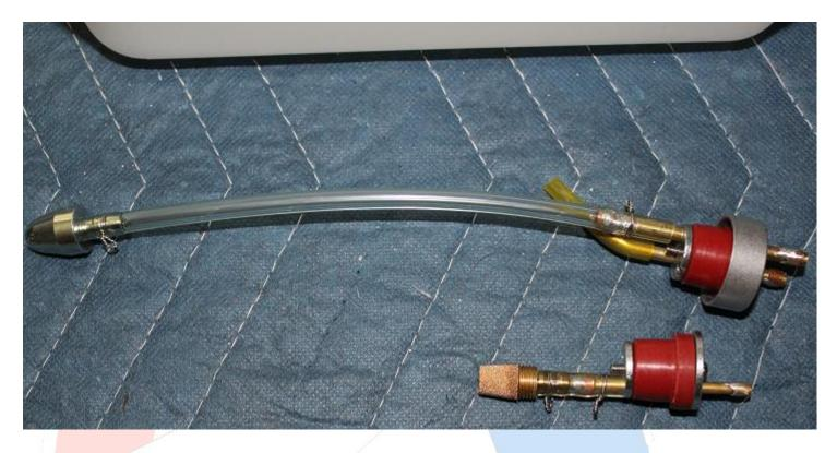
Fuel Tank Tip. If you can't see the vent line and want to see how close it is to the top of the tank, place a flashlight behind it and look though the opposite end. You can accurately see how much wasted fuel space you will have before the fuel spills over.
