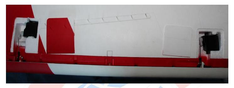
The leading edge flap or slat deflection is about .75 inch or 19mm Max deployment. You want to make sure both are as close as possible to each other on both wings. For takeoff flap, we also used 9mm or .35 inch of slat deployment and 19mm or .75 inch with full flaps down.
