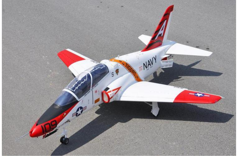
CG 178mm (7 inches) from leading edge at root of wing to fuselage. Ailerons Low 10mm / .40 inch Mid 12 / .47 inch High 14mm /.55 inch. Flaps TakeOff 24mm Landing 40mm Elevator low rate 19mm / .75 inch Mid 23mm / .90 inch High 26mm / 1.02inch. Rudder Low 26mm / 1 inch High 38mm / 1.5 inch Airbrake low 50mm high 85mm (do not operate at high Speed)
