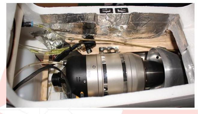
My homemade smoke injector coming off the back of the tailpipe, the glare from the flash makes the tailpipe look as if it was painted grey. If you make your own like this one, make sure it sprays the smoke oil into the exhaust and does not try to push the smoke oil across the tailpipe causing it not to burn or turn into smoke.
