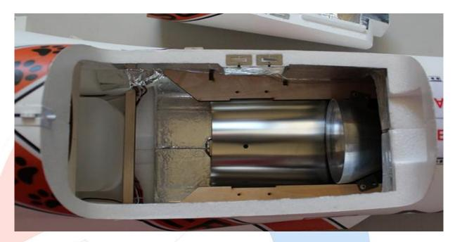
Make sure to check the Turbine to Pipe gap and adjust if needed.
