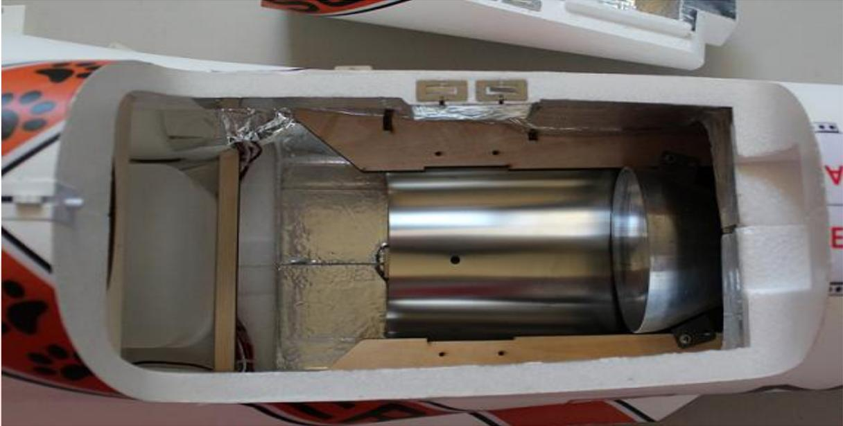
Make sure to check the Turbine to Pipe gap and adjust if needed.
