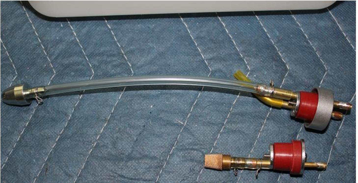
Fuel Tank Tip. If you can't see the vent line and want to see how close it is to the top of the tank, place a flashlight behind it and look through the opposite end. You can accurately see how much wasted fuel space you will have before the fuel spills over.
