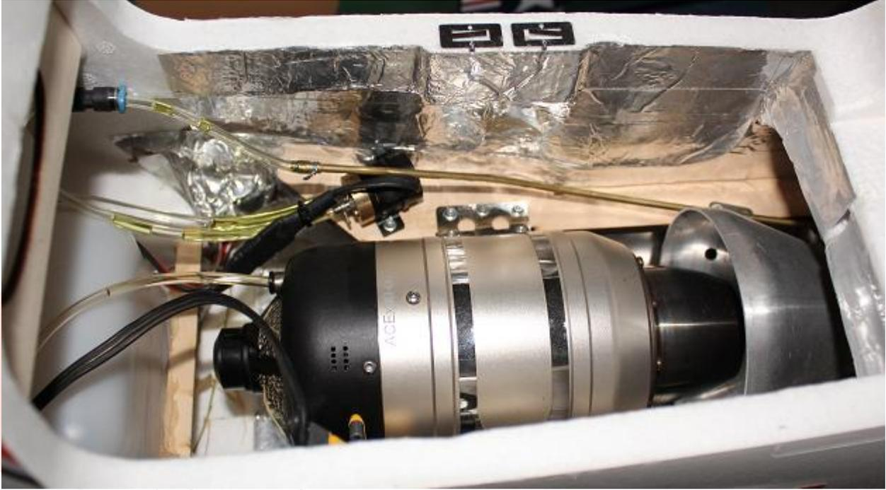
My homemade smoke injector coming off the back of the tailpipe, the glare from the flash makes the tailpipe look as if it was painted grey. If you make your own like this one, make sure it sprays the smoke oil into the exhaust and does not try to push the smoke oil across the tailpipe causing it not to burn or turn into smoke.
