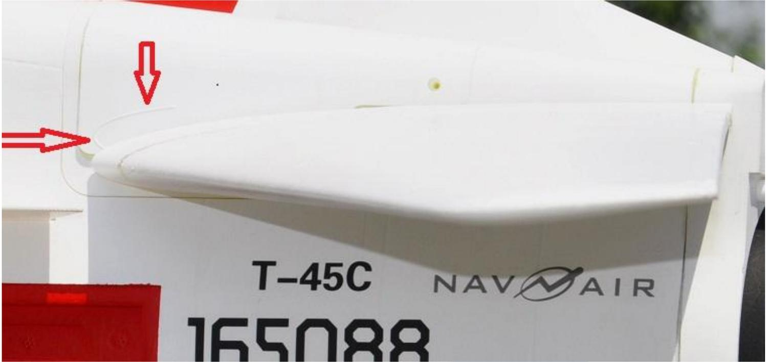
**Vertical Fin / Rudder:** The Vertical fin and rudder are installed on the T-45 by first inserting the carbon spar into the fuselage. The simply match slot in the rudder to the 25g servo already installed for you in the fuselage for the Rudder **Rudder Low 25mm / 1 inch. High 38mm / 1.5 inch**
