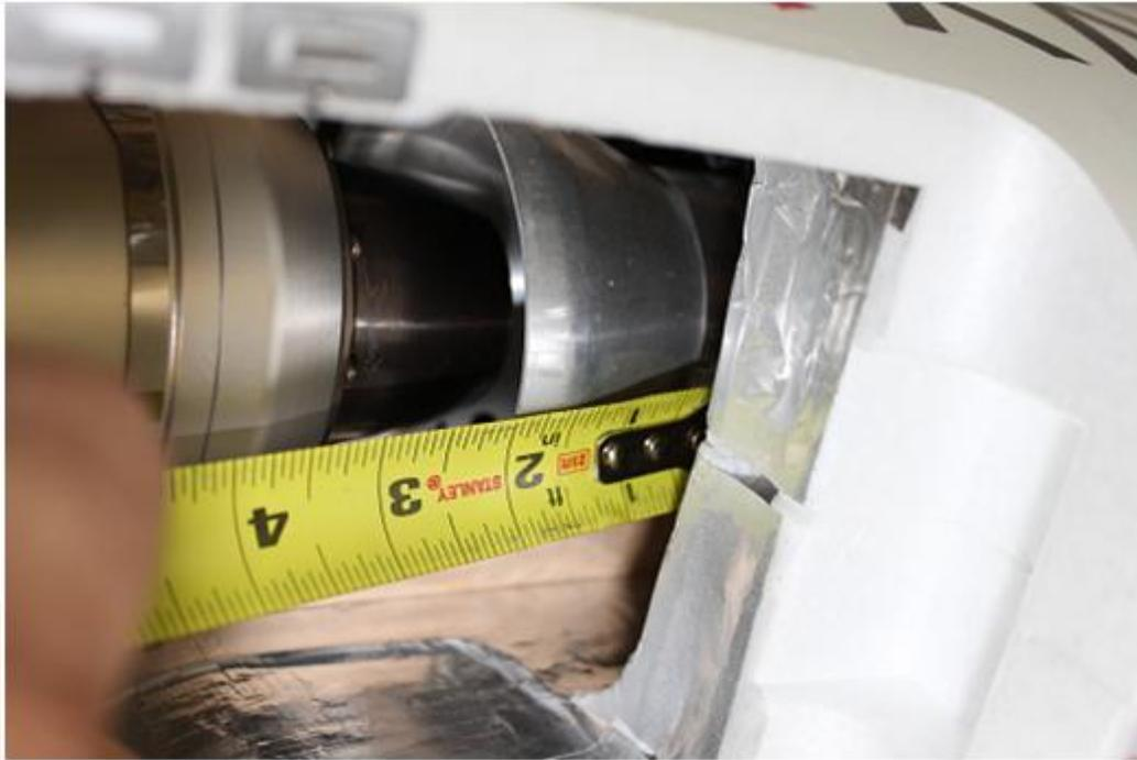
This view of the Turbine installation is to show the Turbine to Tailpipe gap is measured, we check it between the rear of the Turbine and the actual start of the tailpipe NOT the bellmouth of the tailpipe.
