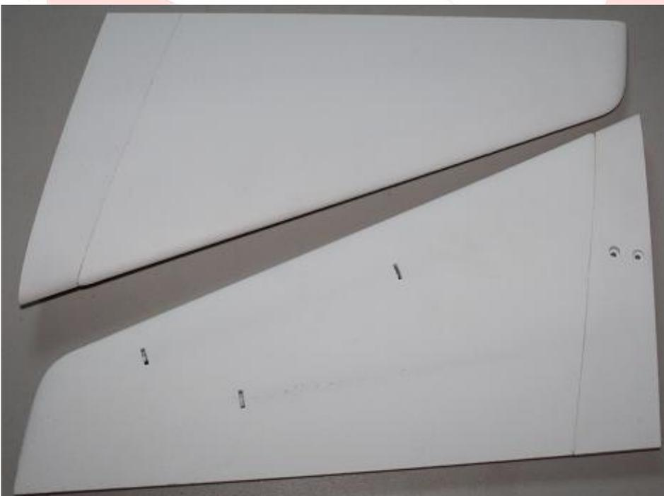
The Elevator cover on the fuselage has a marking for the elevator neutral position, it is the outline of the elevator Airfoil. Simply match the elevator to the airfoil shape and that would be your elevator Neutral Point. Ours needed about 3 clicks of up elevator
