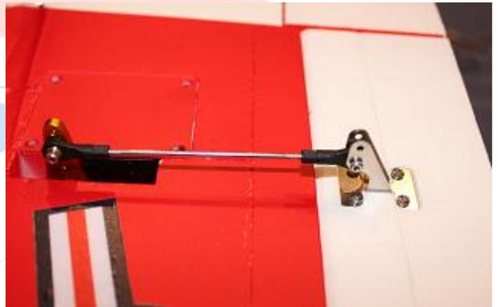
For control rod, you have two options. OPTION #1 Use the third screw from the top on the servo horn and then use the top hole in the control surface. OPTION #2 Use the second hole from the top on the servo horn and then the second hole in the control surface. This gives more of a direct line and allows you to use more of the travel to gain better mechanical advantage and better servo resolution.
