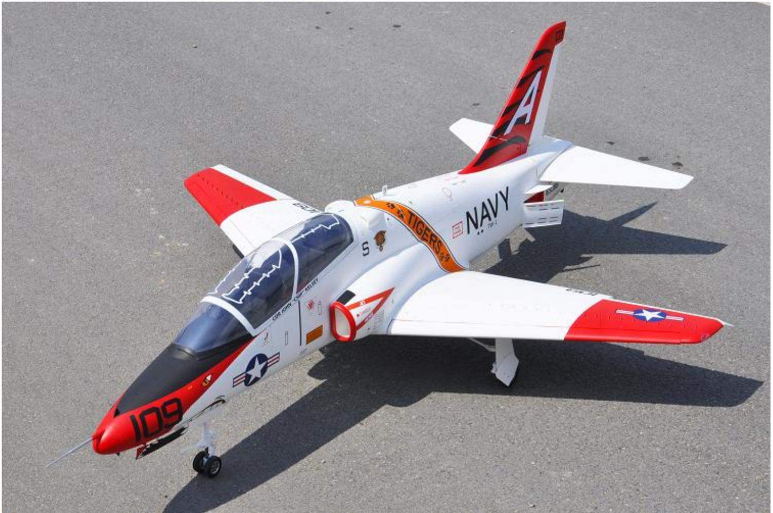
CG 178mm (7 inches) from leading edge at root of wing to fuselage.
