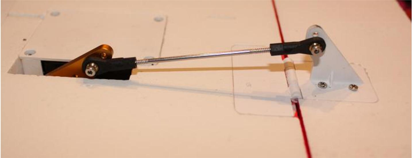
**Leading Edge Flaps / Slats::** The leading edge slats / slats are already installed for you along with the servo and control rods. You need to set your travel throw for that channel so they activate at the same time as the flaps..
