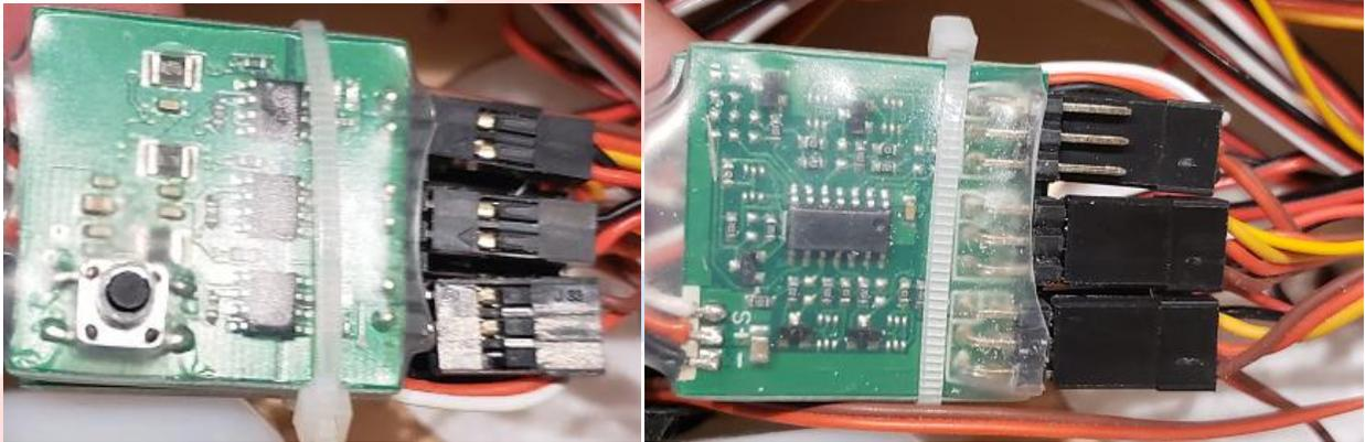
There are two main brake controllers used, a JP basic brake controller and the AG-63 Gyro Assisted Brake controller. The AG-63 will stop your jet by applying brakes and help correct steering if the airplane is not tracking strait (if your airplane is sliding or drifting). We have been using the AG-63 Exclusively in our personal jets and highly recommend this product.
