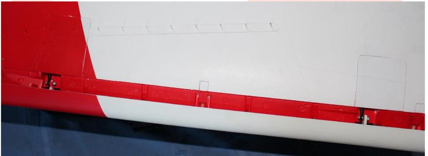
The servo covers are glued and you would have to pry them out, I have removed them here to show you how they are installed at the factory.
