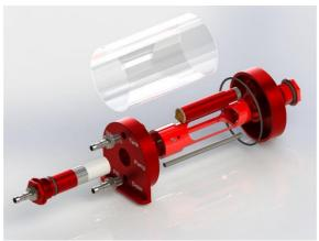
The Centre Pick-Up Tube simply unscrews from the front face of the iTrap giving access to the *SS Super-Flow Sintered Diffuser*. This in turn unscrews from the Feed Tube and can be washed and blown out using an air gun from the inside.
