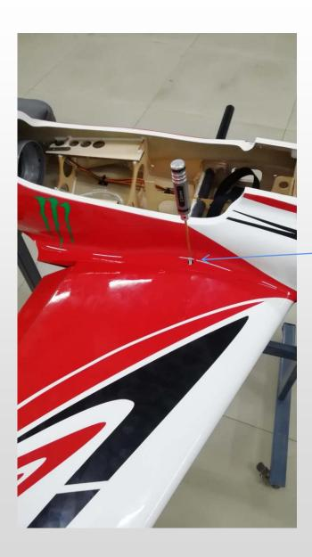
Fixing with M4x25mm inner hexagon screws, Each wing have one screw
