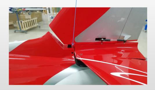
Fixing horizontal tail with 4EA M4x35mm screws, this side and another side both have 2EA screws.
