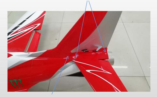
Use 2.5mm inner hexagonal screwdriver to tighten fixing screws for Vertical fin clamp
