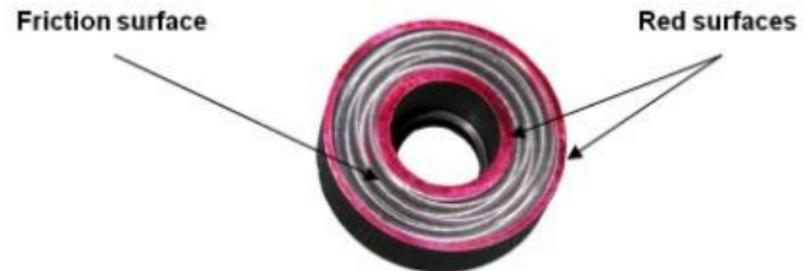
It is advisable to keep clean the grooves of brake disk and the friction surface of the electromagnet, to maintain proper system operation.
